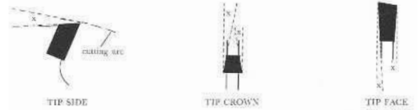
FIG 5. The supporting body of the cutting tip is 'relieved' or ground back (X) so that only the cutting edge itself makes work contact
